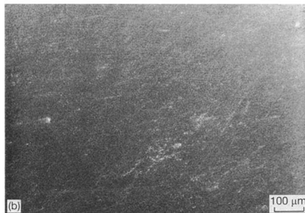
Figure 1 Scanning electron micrographs of (a) pure Cu and (b) DS Cu after polishing. \times 100 .
